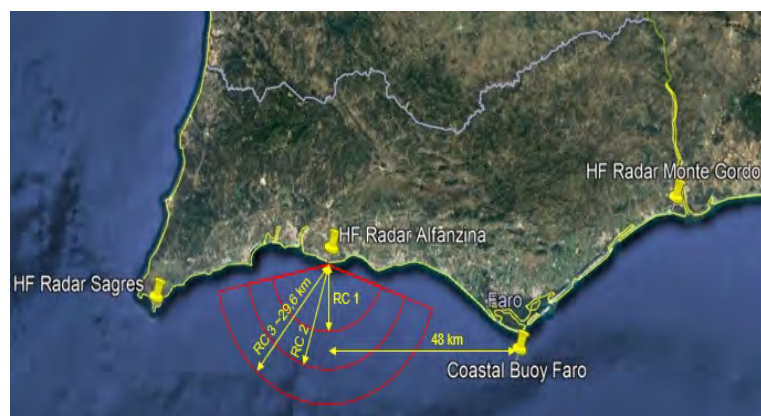
Figure 2: Representative HF Radar range cells, real radar range and distance from the Faro coastal buoy.
